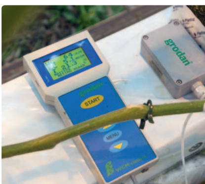
New hygrometer by Grodan. Two pins with a sensor penetrate into a mat in which the plant is rooted. The sensor measures humidity and nutrients in the mat.
